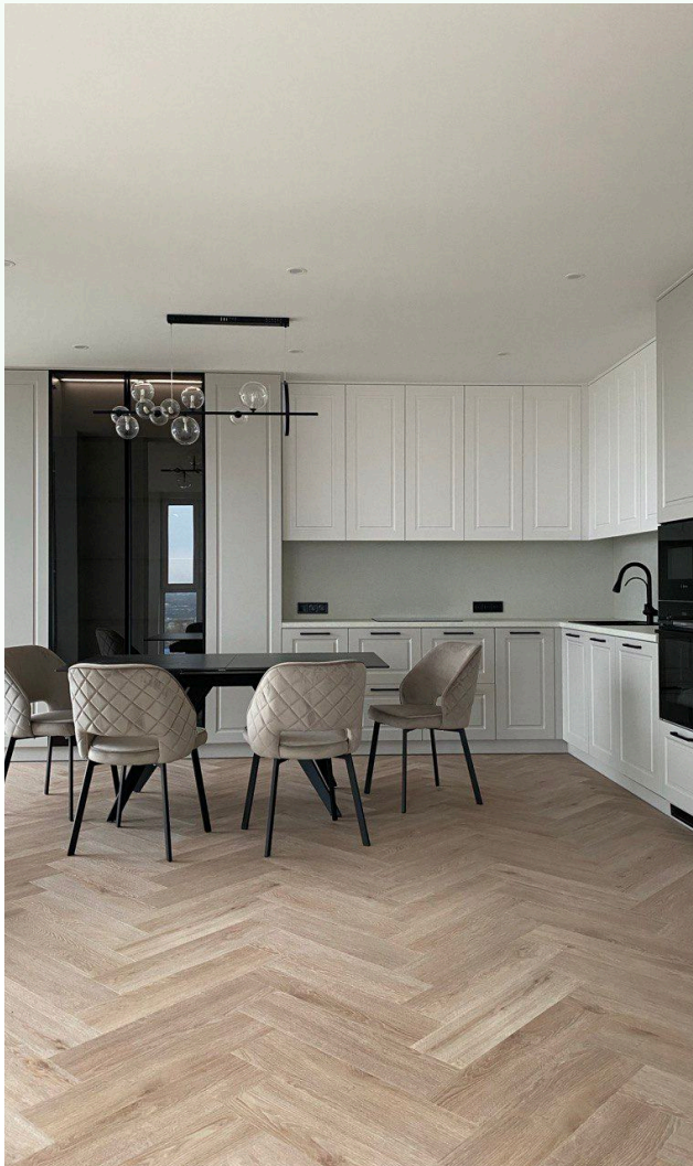
The kitchen is made with facades made of painted MDF with milling. The countertop and wall panel are made of chipboard made in Italy by ARPA. The fittings are mixed by Blum+Muller.
